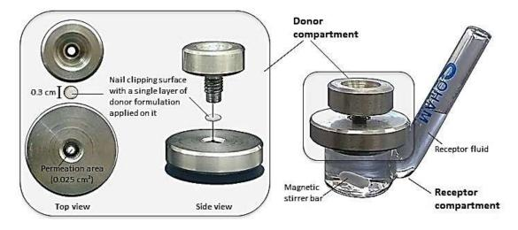
**Fig. 4.2** Modified Franz diffusion cell used for permeation studies. The donor compartment was made from steel and the receptor compartment from glass.
