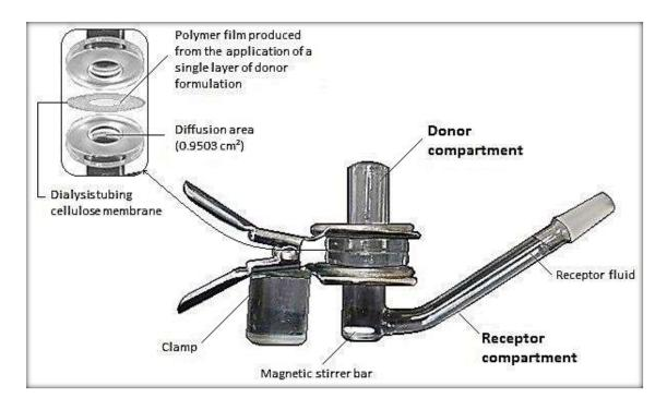
Fig. 4.1 Franz diffusion cell set up for release studies. The cellulose membrane was only used to support the Curanail<sup>®</sup> film. UV-cured films did not need any support.
