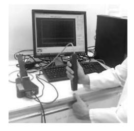
Fig. 3.2 Photographic image of the TOWL instrument (Aquaflux) used to conduct film occlusivity tests.
