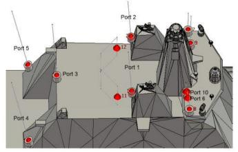
Fig. 1. The various numbered antennas operating at High Frequency (HF) and lower part of Very High Frequency (VHF) on the FPS, shown on the CST model of the main superstructure.
