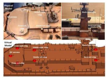
Fig. 8. Locations of the antenna pairs investigated on the 1:50 scale models of the Type 22 Bach II Frigate.
