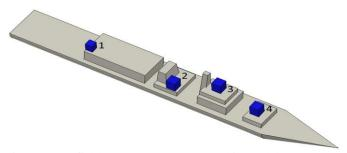
Fig. 3. Near-field sources on a Type 23 ship model.
