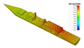
Fig. 4. Distribution of surface current due to emissions of near-field source 1.
