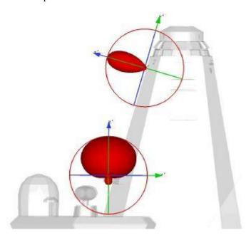
Fig. 5. Far-field antenna sources for INMARSAT C transmit antenna model and an element of the Iridium array satellite receive antenna model on the FPS model.
