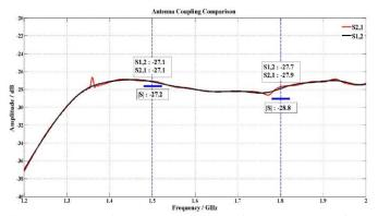
Fig. 15. Result for cross-validation of the A-Solver of the CST MWS against the T-Solver of the CST MWS for a horn antenna and a biconical antenna.
