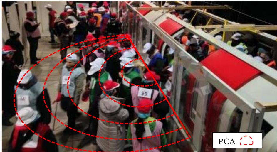
Figure 1. PCA divided into layers at PAMELA (with PEDs)
