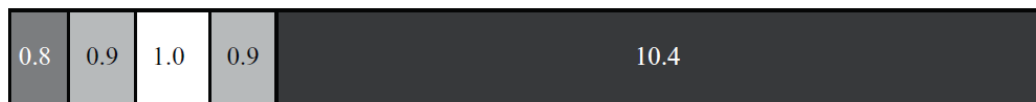
Figure 1.1: Cross section through the typical layers in a bag. Polyester (dark grey), bonding agent (light grey), Ethylene Vinyl Alcohol (white), bonding agent and Polyethylene (black). Taken from Brecht (2009).
