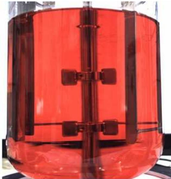
Figure 2.7: NewBrunswick BioFlo 110 stirred tank reactor.
