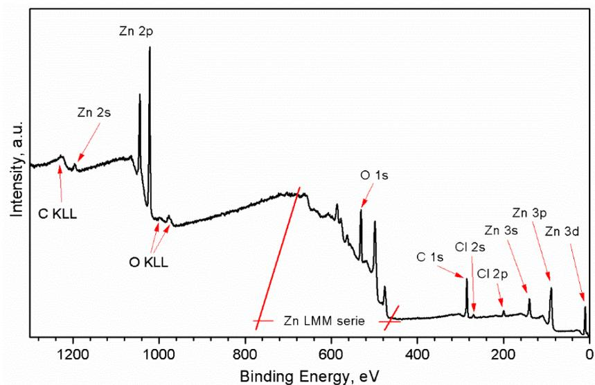
**Figure S3.** Survey XPS spectra for the aerosol-assisted chemical vapor deposited ZnO rods.
