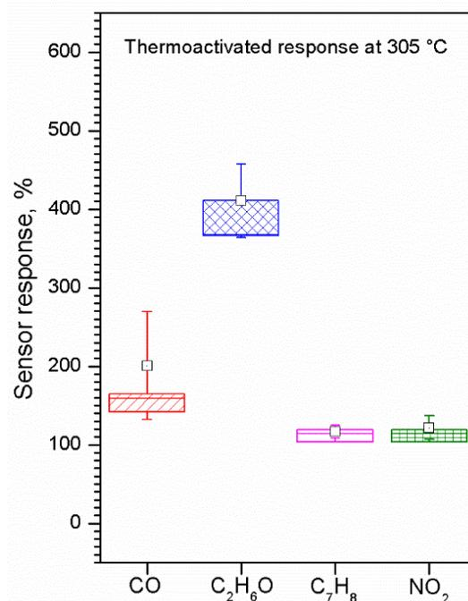
**Figure S6.** Box plots of the sensor response to 100 ppm of CO, C<sub>2</sub>H<sub>6</sub>O, C<sub>7</sub>H<sub>8</sub> and NO<sub>2</sub> obtained from the thermoactivated tests at 305 °C. Each box displays the median, mean, and upper and lower quartiles (first and third) of the respective distribution. Box whiskers indicate the standard error.
