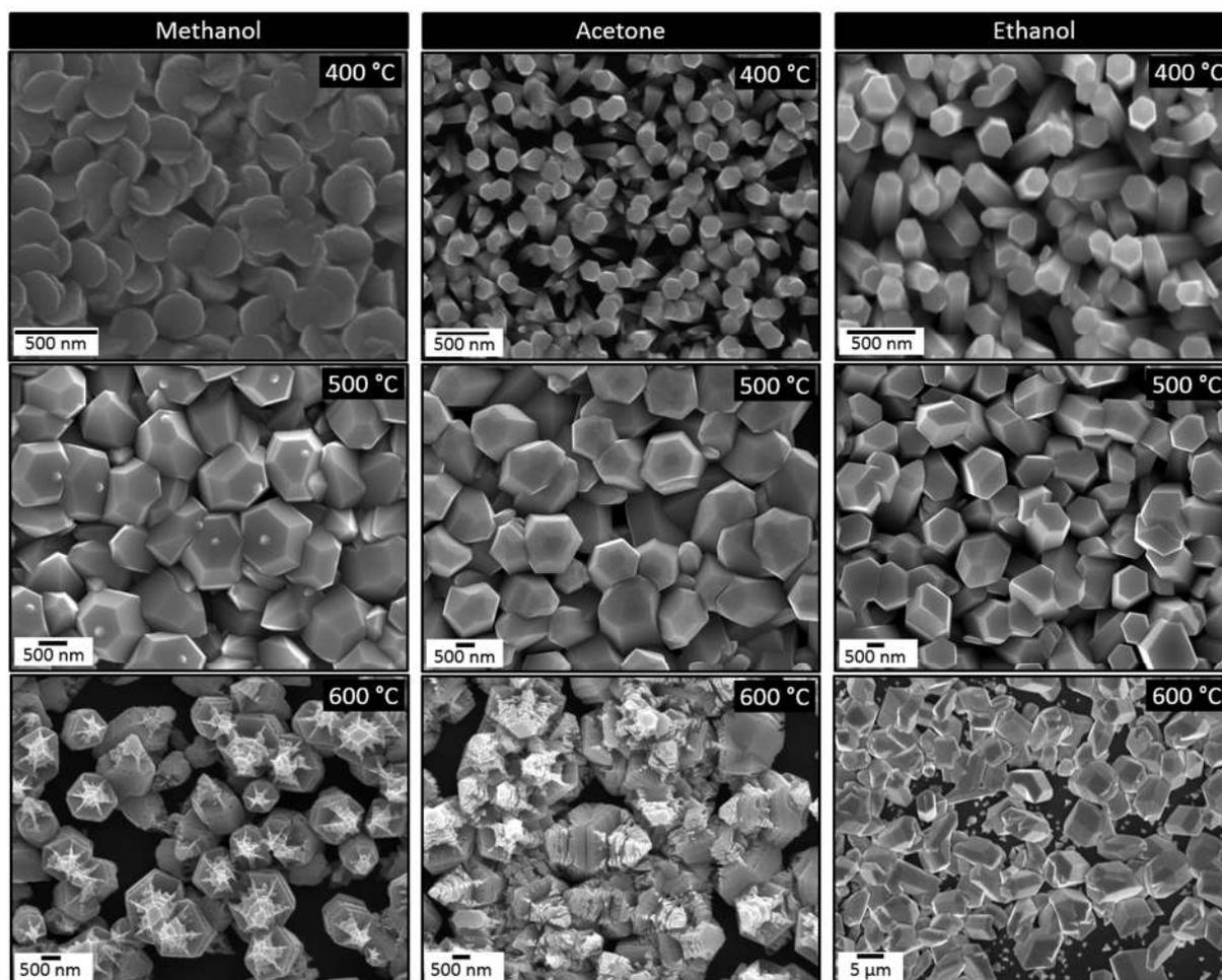
**Figure S1.** Typical SEM images of the aerosol-assisted chemical vapor deposited ZnO films grown at different temperatures either on silicon or glass substrate.
