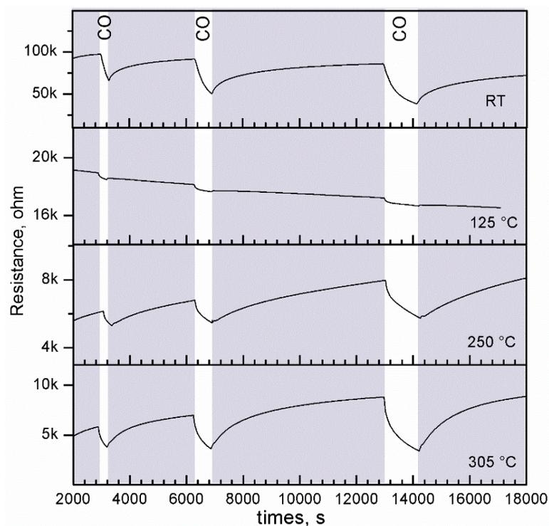
**Figure S5.** Film resistance changes towards 100 ppm of CO at RT (photoactivated response) and 125 – 305 °C (thermoactivated response).
