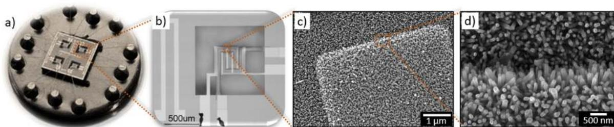
**Figure S4.** Photograph of the 4-microsensor array mounted on a standard TO8- package (a), view of a single microsensor platform (b), and SEM images at low (c) and high (d) magnification showing one of the electrode-ends of the microplatform and the ZnO rods grown onto it.
