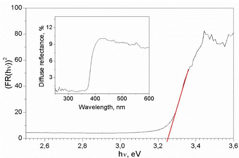
**Figure S2.** Diffuse reflectance spectra of the ZnO rods (inset) and estimation of the optical bandgap using the Kubelka-Munk method.
