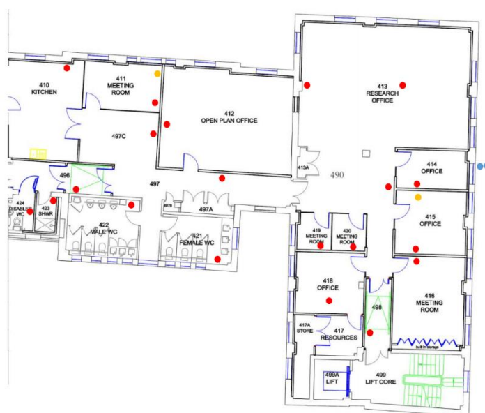
Figure 2: Logger placement. Red dots indicate internal loggers, orange dots loggers near air conditioning units, and blue dots indicate external loggers. (Sang, 2015)
