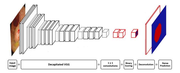
Figure 2: Illustration of a FCN-VGG for polyp detection. The decapitated VGG consists of the VGG network architecture<sup>11</sup> without the fully connected and scoring layers. The layers in red color are the ones that were added to form FCN-VGG. Image adapted from.<sup>12</sup>
