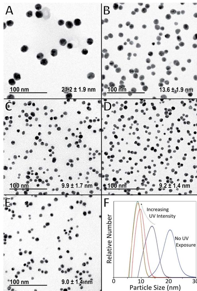
Fig. 3 TEM micrographs of AuNPs produced with different intensities of UV light at constant UV residence time (10 s), growth residence time (20 min) and growth temperature (80  $^{\circ}\text{C}$ ). (A) No UV lamps used, (B) one lamp, (C) two lamps, (D) three lamps, (E) six lamps and (F) particle size distributions obtained from DCS (normalised by area under each curve).
