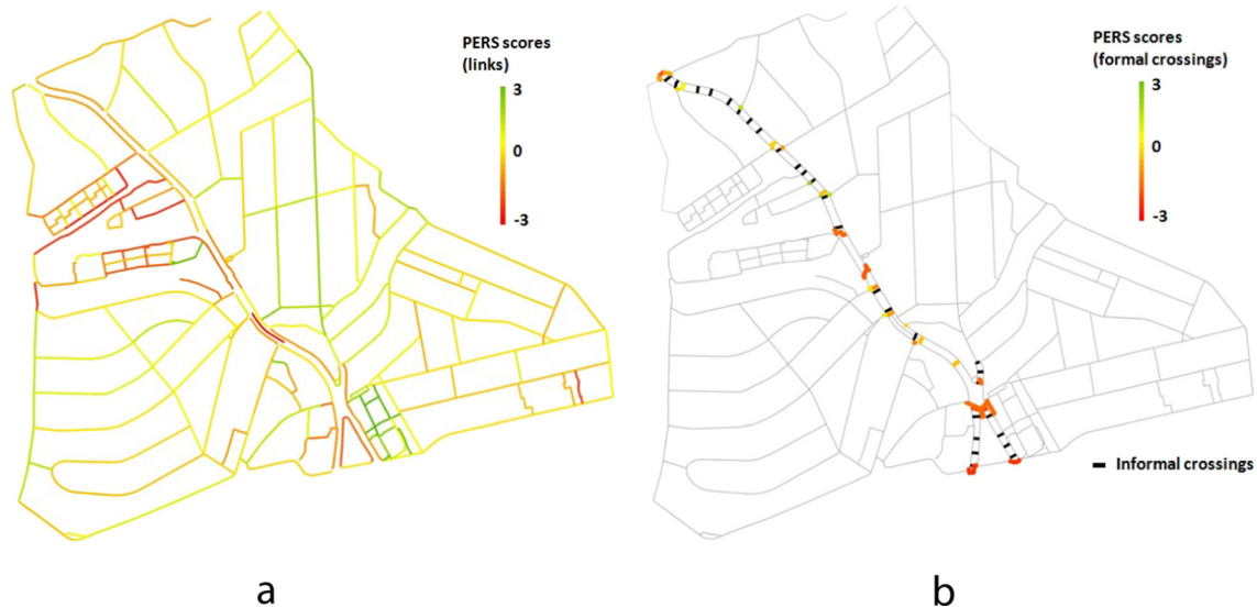
Fig. 6. Pedestrian Environment Review System (PERS) scores of links (a) and crossings (b). Note: The higher the score, the better the pedestrian environment.
