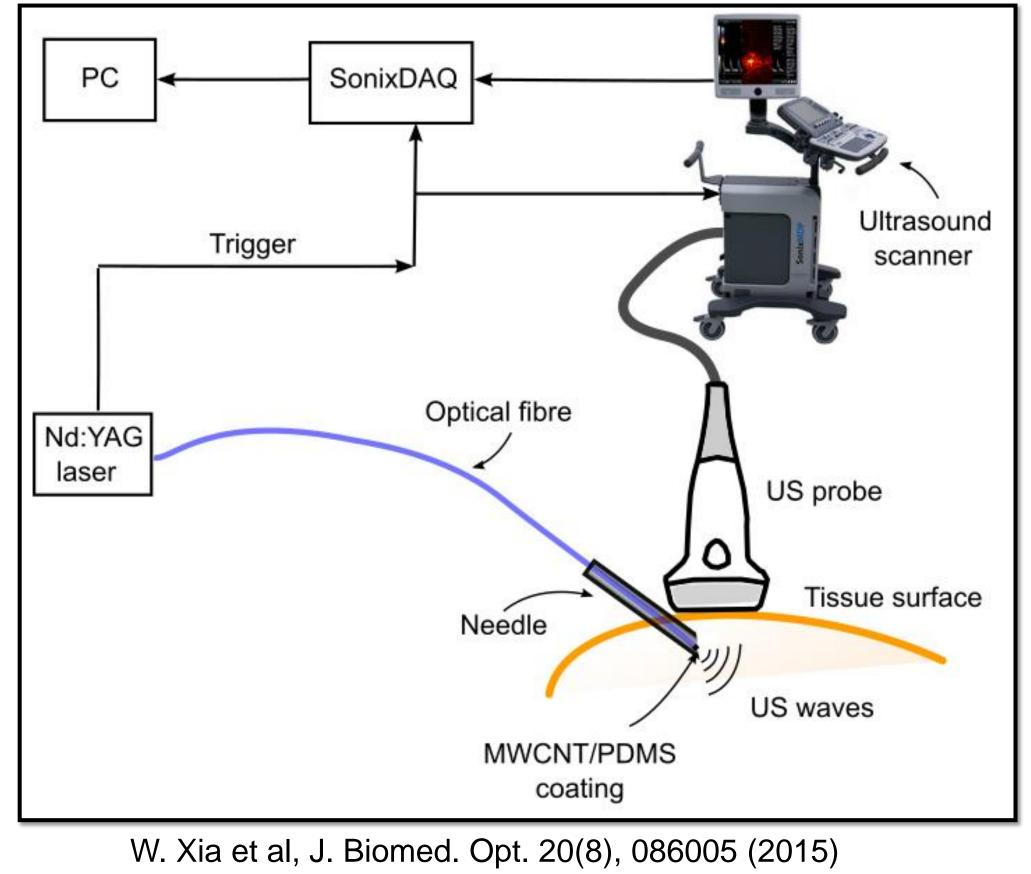
PDMS coating on the tip of the light delivery fibre embedded in a needle Clinical US with 14–5
