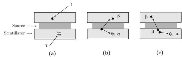
Figure 4: Illustration of the possible sources of background: (a) random coincidences due to the  $\gamma$  flux, (b)  $^{212}\text{Bi}$  or  $^{214}\text{Bi}$  contamination on the surface of the scintillators, (c)  $^{212}\text{Bi}$  or  $^{214}\text{Bi}$  contamination in the volume of the scintillators.
