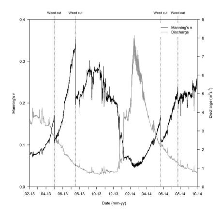
**FIGURE 2** Calculated Manning's n roughness coefficient and discharge inputs for the MIKE 11 hydraulic model for the river Lambourn
