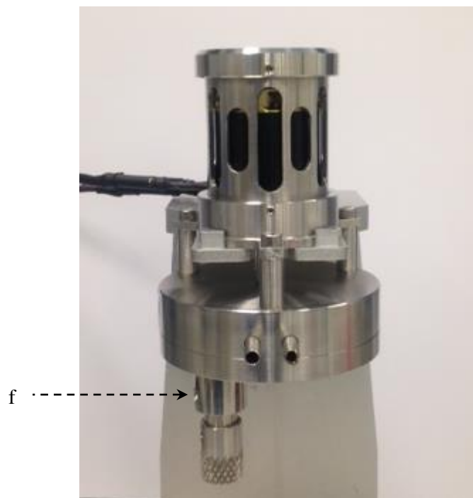
Figure 2-5: a) Schematic diagram of the shear device used for USD centrifugation and shear evaluation of microalgal cells and flocs: a = motor, b = cooling port (water inlet and outlet), c = 1 mm, d = 40 mm, e = 50 mm and b) photograph of the device; f = feed inlet/outlet.
