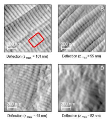
**Figure 4** AFM deflection images of untreated rat tail tendon (panel A) and unaged parchment sample (B-D) prepared using three different methods. Panel B shows an AFM image of a parchment fibres scraped from the flesh side, panel C shows an AFM image recorded directly on the flesh side and panel D shows an AFM image of a cross-section prepared using a cryotome. The red rectangular highlights the D-banding periodicity. The images are from de Groot's PhD thesis (23).
