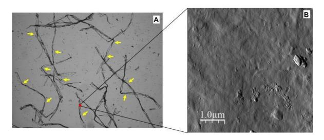
**Figure 8** Panel A: Bundles of collagen fibres extracted from the historical parchment for The Kew National Archives (London, UK). The image was acquired with a light optical microscope at a magnification of 100x and the yellow arrows highlight the twist and pearls structure. Panel B: AFM deflection image acquired on a collagen fibre showing a damage morphology appearance. The collagen scaffold in this location is characterised by the complete loss of its characteristic features.
