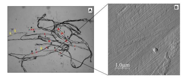
**Figure 6** Panel A: Bundles of collagen fibres extracted from new parchment hide. The red dots indicate the area analysed by AFM, whilst the yellow arrows highlight the twist and pearls structure. The image was acquired with a light optical microscope at a magnification of 100x. Panel B: AFM deflection image acquired on a collagen fibre showing an intact-like appearance. The collagen scaffold is characterised by fibrils aligned in register with a visible D-banding.
