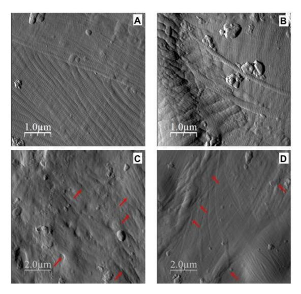
**Figure 9** Representative AFM deflection images for the historical parchment sample, showing intact banded collagen fibril aligned in register (panel A), disruption of the well-organised collagen structure and the wrinkling of the surface (red arrows).
