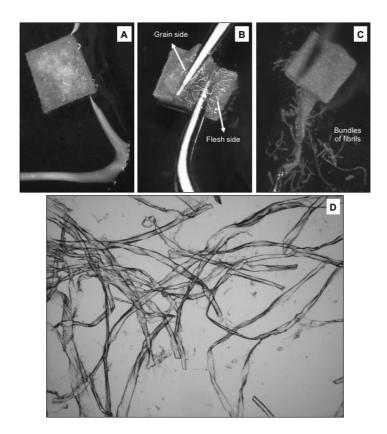
**Figure 3** Microsampling for the extraction of collagen fibres from parchment. (A) soaking of parchment in water. (B) separation of grain side from the flesh side with the help of sharp tweezers. (C) Pulling out of bundles of fibres from the flesh side. (D) Extracted bundles of collagen fibres, still in water, observed under an optical microscope at a magnification of 100x.
