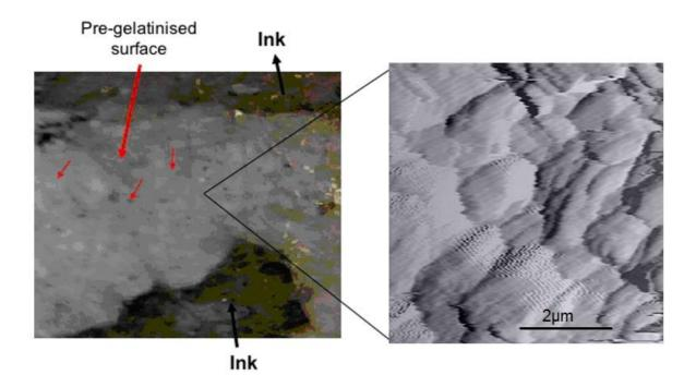
**Figure 11** The handheld digital image accessory shows the parchment surface in the area raster-scanned with AFM: the related image (on the left, magnification 50x) shows an area on parchment between two letters, characterised by a pre-gelatinised state. This is confirmed by the related AFM image (on the right, scan size  $10~\mu m$ ) where the collagen scaffold is characterised by a complete loss of its typical structure, similar to Figure 7c
