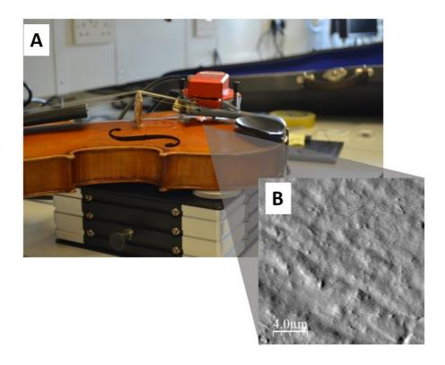
**Figure 2** Nanosurf Easyscan 2 AFM head on violin placed on an anti-vibration table (A) and AFM image of the surface of the violin (B)
