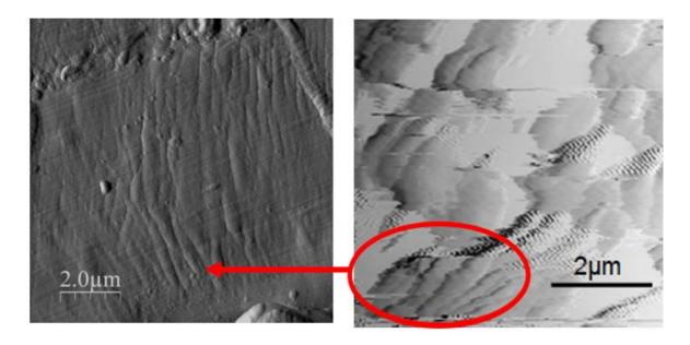
**Figure 12** Example of damage (folding or wrinkling) as seen in image recorded from an extracted fibre (on the left) and in image directly recorded on parchment surface of similar dimension and showing a similar folding pattern (on the right, highlighted by the red circle, scan size 5  $\mu$ m). AFM image also shows problems with loss of contact between tip and sample in certain areas.
