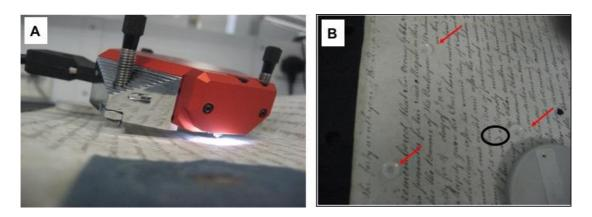
**Figure 10** Panel A shows the setup of the EasyScan with the AFM safely placed directly on the parchment document thanks to the use of soft plastic supports to protect the document from damage due to AFM moving (highlighted with red dots in panel B). The black circle in panel B shows the area imaged with AFM
