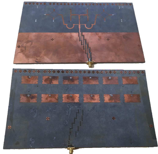
Fig. 9. Single element phased array antenna prototype. The top image shows the phased array feed network and the bottom picture indicates the phased array radiating elements
