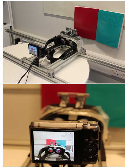
Figure 2: Latency estimation rig. Top: Showing HMD and camera strapped to a sled that is mounted on rails. Bottom: Showing the camera on the rig capturing both the red/blue target on the wall and the distorted view of the red/blue target through the lens.
