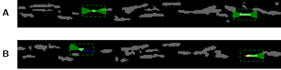
Figure 3.3: Custom restrictions to particle linking. A custom set of cost functions for uTrack was developed in order to improve performance when tracking mitochondria. A: Particles without a known trajectory, or slowly moving particles, can connect to particles on both sides within a maximum displacement (dashed line, arrow) and a given angle \alpha from the horizontal line. B: Particles which are moving with a known velocity can only connect to new particles close to their current position (stopping) or within \alpha relative to their current velocity.
