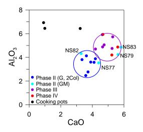
**Figure 9.**Al<sub>2</sub>O<sub>3</sub>versus CaO plot for the lead glazes. We can see that the Phase IIG and 2Col lead glazed wares contain less Al<sub>2</sub>O<sub>3</sub> and CaO than those of Phase III and IV. Among the lead glazes present in the undecorated side of the tin glaze GM decorated wares, two samples, NS83 and NS79 group with the Phase II group while NS77 abs NS82 with the Phase III and IV group.
