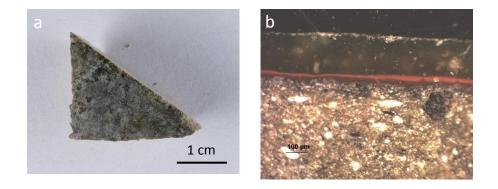
**Figure 5.** a) Standard and b) Dark Field Microscopy image of NS121 green glaze (Phase II) showing a red band closer to the glaze ceramics interaction layer.
