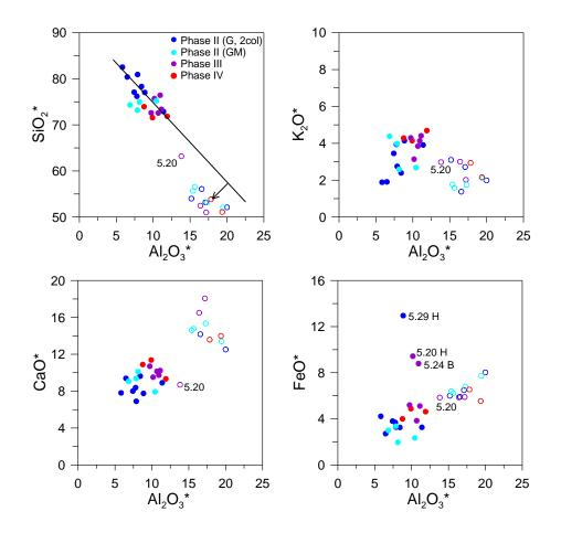
**Figure 10**.Comparison between the chemical composition of the ceramic pastes (open dots) to those of the lead glazes renormalized after removing PbO and the colourants CuO and MnO<sub>2</sub> (solid dots).
