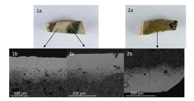
**Figure 6.** 1a) Standard picture of tin glaze with decoration in brown and green in Sample NS83. 1b and 1c) SEM-BSE images of the white and green glazes of the sample. 2a) Standard picture of the reverse glaze of Sample NS83. 2b) SEM-BSE image of the reverse glaze of the same sample.
