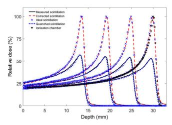
**Fig. 6.** Percentage depth dose curves at 38.94, 46.77, 53.86, and 60.00 MeV, showing (a) the simulated depth dose (blue crosses); (b) the depth dose directly measured by the camera (solid black line); (c) the simulated quenched light output (blue bars); and (d) the measured light output after correction for quenching (red dashes).
