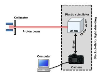
**Fig. 1.** Schematic of the experimental setup. The camera was positioned at 50  $\pm$  0.5 cm perpendicular to the proton beam and data acquisition was performed using a Nikon camera controlled by software on a laptop computer situated outside the treatment room connected via a 25 m USB cable. Black cloth and tape were used to exclude ambient light.
