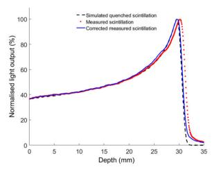
**Fig. 2.** Percentage depth doses shown for data extracted from the photography directly without magnification correction (red dots), simulated light output with quenching (black dashes) and the measured data after correction for magnification (blue line). The agreement between data and simulation improves following the magnification correction.
