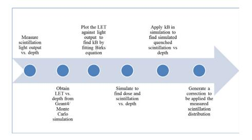
**Fig. 3.** Summary of the quenching correction procedure.
