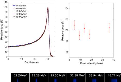
**Fig. 8.** The response of the scintillation detector system after delivering 4.5 Gy at different dose-rates for a 60 MeV proton beam. Vertical bars on the right hand graph give the measurements error.
