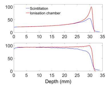
**Fig. 4.** Depth-dose profile comparisons between ionization chamber measurement and measured scintillation light for a pristine Bragg peak (top) and a spread out Bragg peak (bottom).
