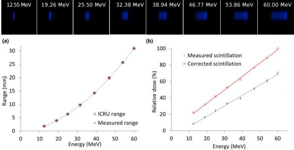
**Fig. 9.** Images obtained by the scintillation detector system show (a) The variation in range with the proton energies used in this study (b) The impact of different proton beam energies on the response of the detector system.
