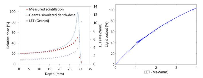
**Fig. 5.** (a) LET values simulated by Geant4, depth dose profile simulated in Geant4, and the measured scintillation light distribution as a function of depth for a 60 MeV proton beam in a BC-408 scintillator (b) The measured scintillation light vs simulated LET for the 60 MeV proton beam (note that the highest LET points do not contribute to light output as they occur beyond the Bragg peak).
