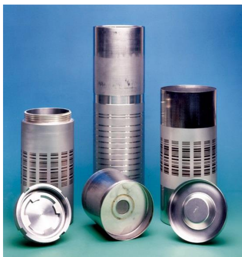
Figure 3.1 Steel cans used for the storage of plutonium dioxide powder, from 76
