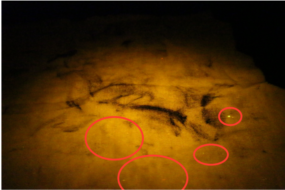
Figure 16. A swatch of fabric seeded with GSR from a SA80 visualised under blue-green light
