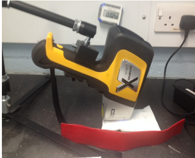
Figure 14. The experimental setup of the p-XRF experiments
