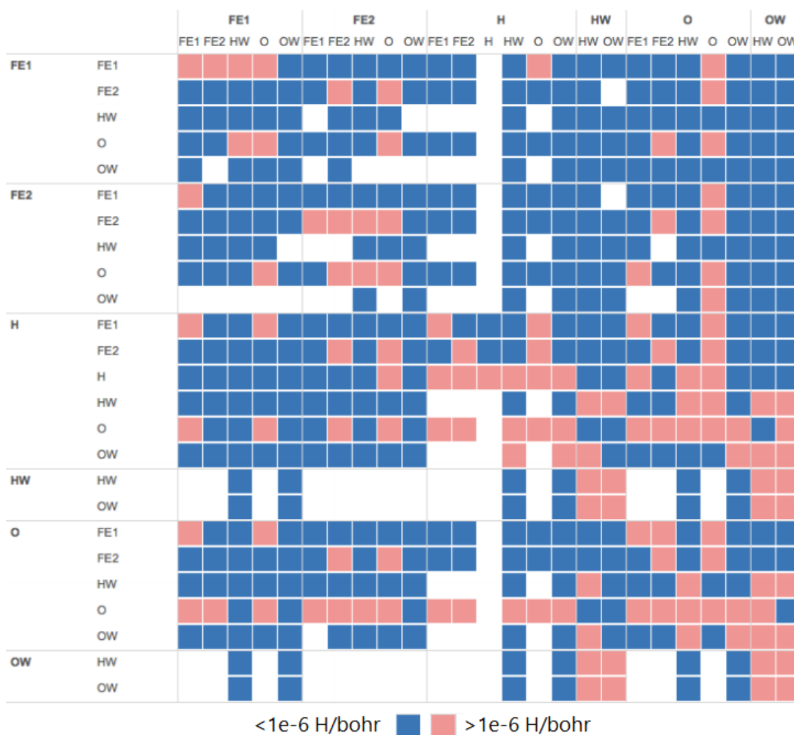
▲ Figure 4.1 – Maximum absolute force contribution resulting per atom kinds of the four orbitals involved. In the setup in question, there are six atom kinds: Fe1 and Fe2 (iron atoms that differ by their majority spin in the antiferromagnetic spin pattern of hematite), H and O for hydrogen atoms and oxygen atoms within or at the surface of hematite, as well as HW and OW for hydrogen atoms and oxygen atoms in bulk water. Coloured cells denote combinations where the maximum force contribution is above (red) or below (blue) the threshold of 10^{-6} H/bohr. Empty or missing cells mark combinations that did not occur in this particular MD step, likely due to exclusion during the overlap screening or due to symmetry considerations. All calculations in the blue cells include 23% of the total ERI recorded.
