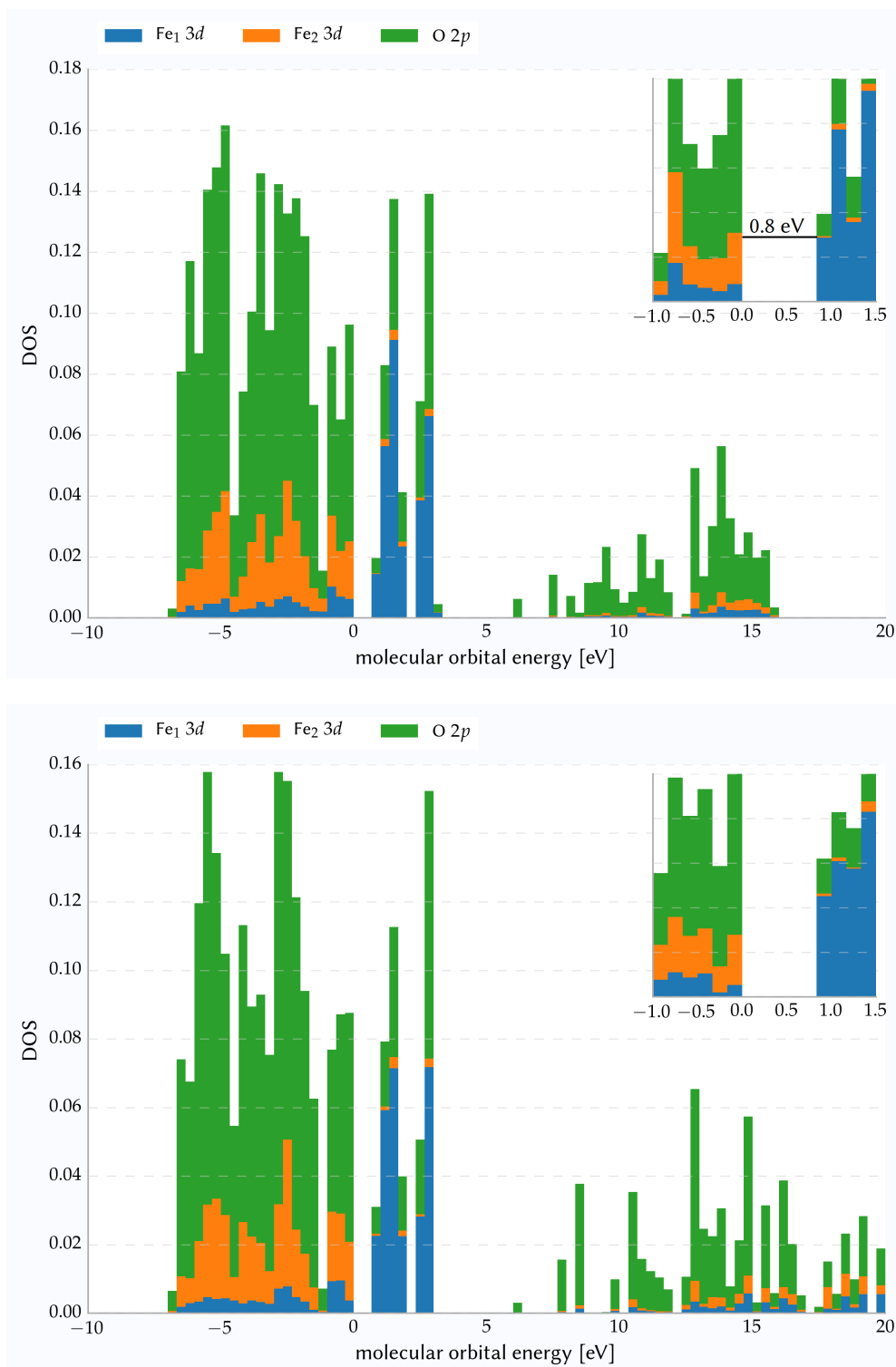
▲ Figure 2.7 – Projected \alpha density of states for the three atom kinds for the PBE functional. Beta spin iron is denoted as \text{Fe}_1 , alpha spin iron as \text{Fe}_2 . Only 3d (iron) and 2p orbitals (oxygen) contribute to this histogram. Orbital energies are shifted such that the Fermi energy is at zero molecular orbital energy. The inset shows the region around the band gap at the \Gamma point. While both histograms are normalised, the bins are different for the main graph and the inset. Calculations done with DZVP-MOLOPT-SR-GTH basis set. Top: 270 atoms ( 3 \times 3 \times 1 unit cells). Bottom: 120 atoms ( 2 \times 2 \times 1 unit cells).
