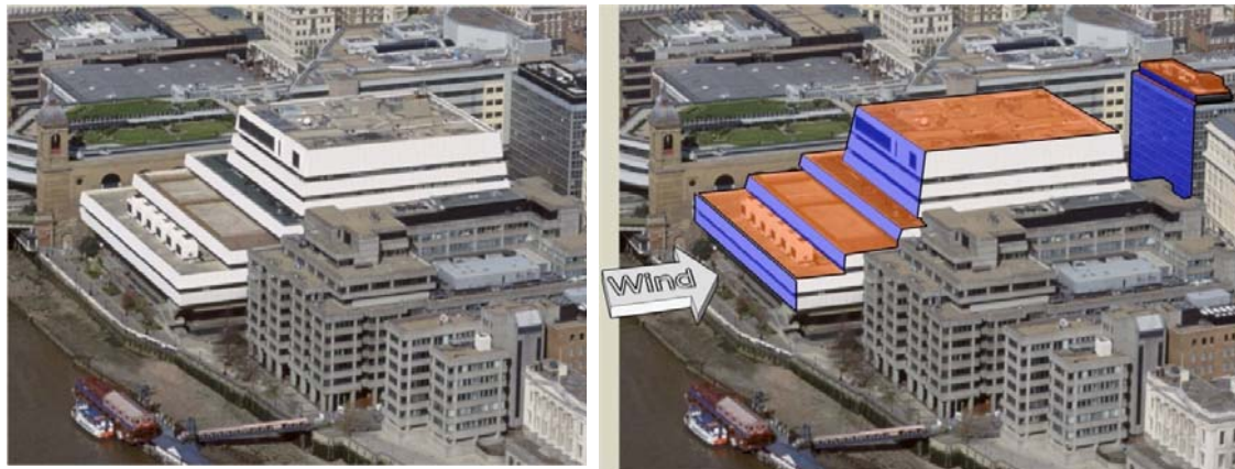
Fig. 4 - An example of A_F (blue) and A_P (orange) illustrated for a specific wind direction on some London buildings, showing how an urban area can be much more complex to work with in reality.
