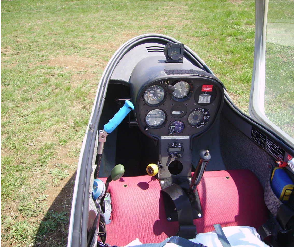
Front seat of a two-seater glider in Bilonia. It shows the instrument panel, the stick (black in the centre), the yellow knob used to release the tow rope, the trim lever (green, on the left side), the airbrakes lever (light blue, on the left side), the microphone (right side).
