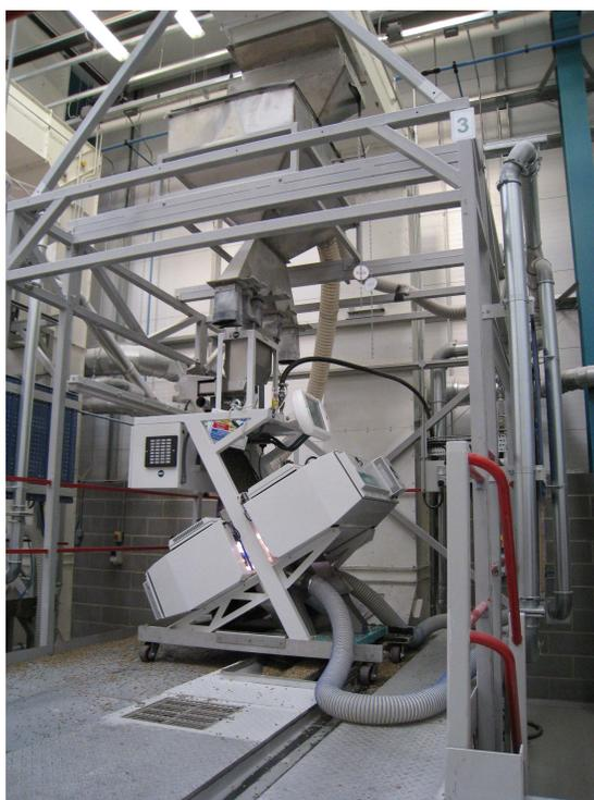
Figure 5.21: Buhler Sortex Z1 sorting machine and recirculation rig. Picture ©copyright Buhler Sortex Ltd, 2008. Printed with permission.
