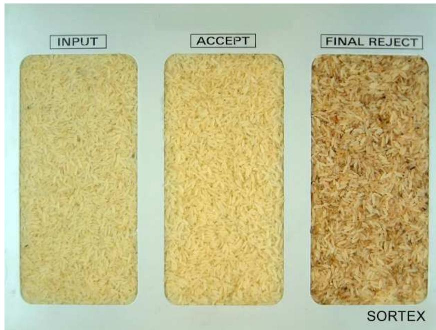
Figure 1.3: Input, Accept and Reject Samples for White Long Grain Parboiled Rice using a Buhler Sortex Z-series machine. Picture ©copyright Buhler Sortex Ltd, 2008. Reprinted with permission.
