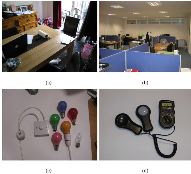
Figure 4.5: Locations and equipment used to create different lighting conditions. 4.5(a) shows the naturally lit lounge and 4.5(b) shows the office lit by florescent bulbs. 4.5(c) shows the bulbs and dimmer switch used create local lighting variation, 4.5(d) shows the light meter used to approximately monitor the ambient lighting conditions.
