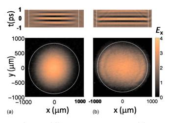
FIG. 3. (Color online) (a) Bottom panel: spatial electric field  $(E_x)$  distribution at t=0 measured at the output of the waveguide using the terahertz near-field probe; top panel: the corresponding space-time map showing the pulse waveform along the horizontal axis. (b) Similar measurements on a waveguide with the same dimensions however without the dielectric layer.
