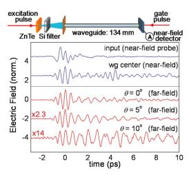
FIG. 4. (Color online) Terahertz pulse waveforms measured in the near-field and the far-field regions. Near-field waveforms are detected by the near-field probe. Angle-resolved waveforms are detected by a photoconductive antenna in the far-field zone. The top waveform shows the input pulse measured by the near-field probe. The schematic diagram shows details of the experimental setup.
