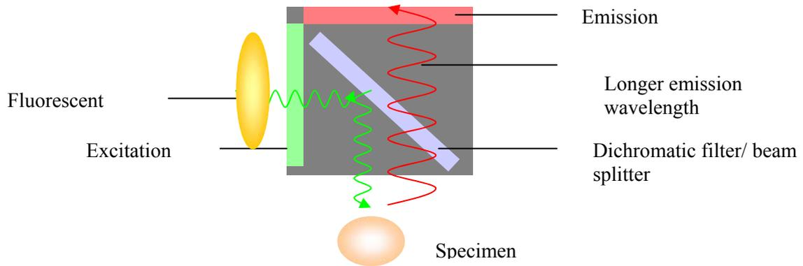
**Fig 2.6 Schema of Filter Block**
