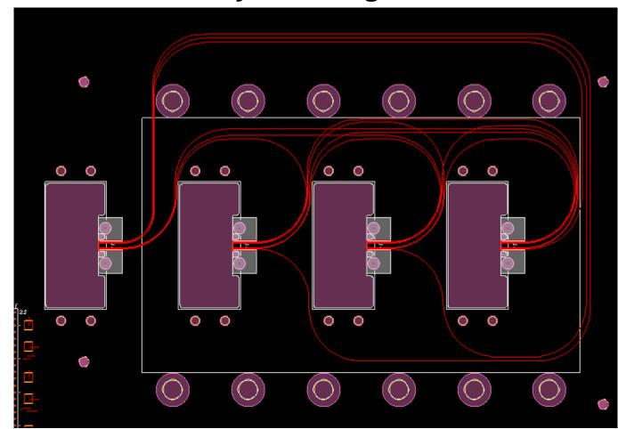
Fully connected waveguide layout using design rules
