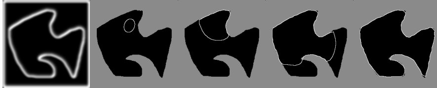
Figure 20 GVF diffusion edgemap (first image) and stages of evolution of the contour to segment a non convex shape by the GVF snake.
