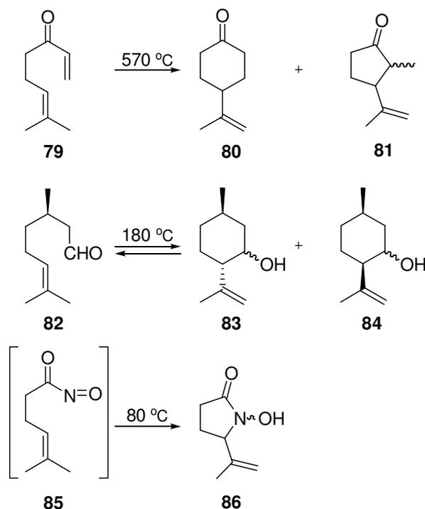
Scheme 26: The acyl nitroso intermediate **85** was thermally released from its Diels-Alder adduct at 80 °C, followed by intramolecular ene reaction.
