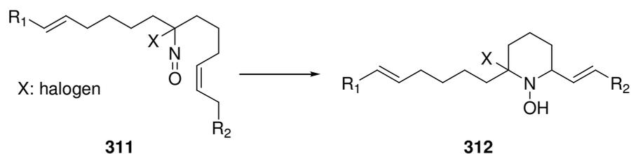
**Step 2** Elimination of hydrogen halide to form a nitron
