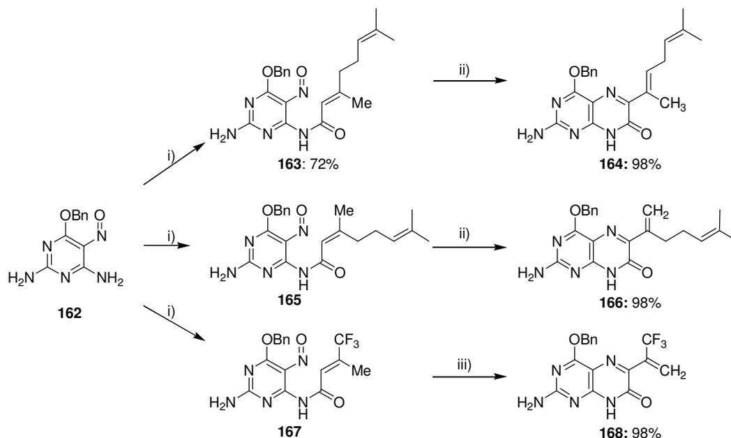
i) 1.3 eq RCOCl, K<sub>2</sub>CO<sub>3</sub>, -18 °C, THF. ii) sol in CH<sub>2</sub>Cl<sub>2</sub>, 4 days. iii) suspension in toluene, 150 °C, 8 h in sealed vial.
