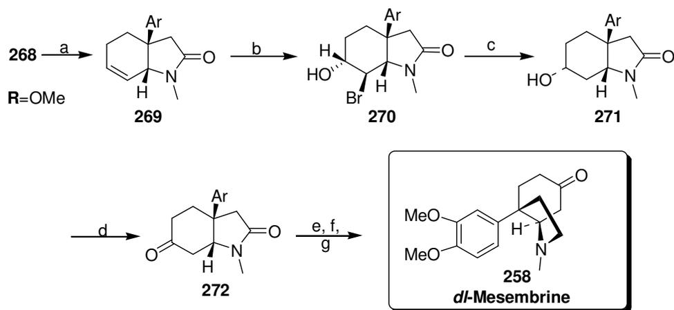
a) NaH, CH<sub>3</sub>I, THF; b) NBS, 4:1 DME-H<sub>2</sub>O; c) (CH<sub>3</sub>(CH<sub>2</sub>)<sub>2</sub>CH<sub>2</sub>)<sub>3</sub>SnH, AIBN, toluene, reflux; d) PCC, CH<sub>2</sub>Cl<sub>2</sub>, 0 °C; e) HOCH<sub>2</sub>CH<sub>2</sub>OH, benzene, reflux, *p*-TsOH; f) LAH, THF, reflux; g) H<sub>2</sub>O<sup>+</sup>
