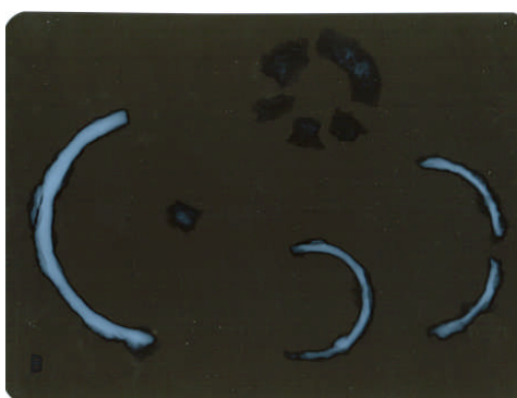
Fig. 5.21 X-ray taken of the objects displaying the level of corrosion affecting the iron metal (X-ray courtesy of Kelly Caldwell).
