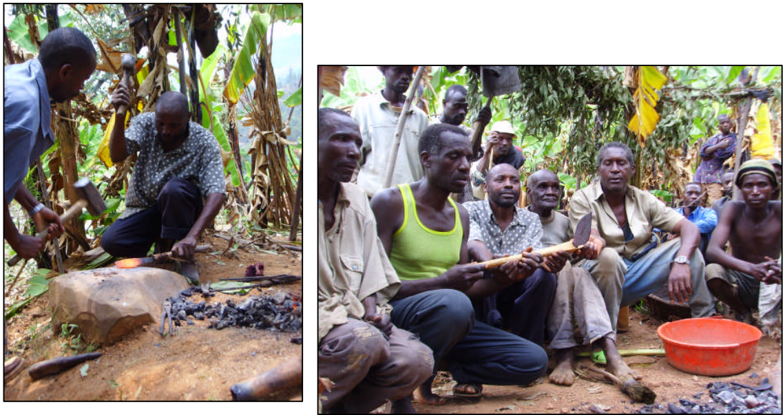
Fig. 2.7 Forging the marriage hoe (left), and the finished product with some of the successful team (right)
