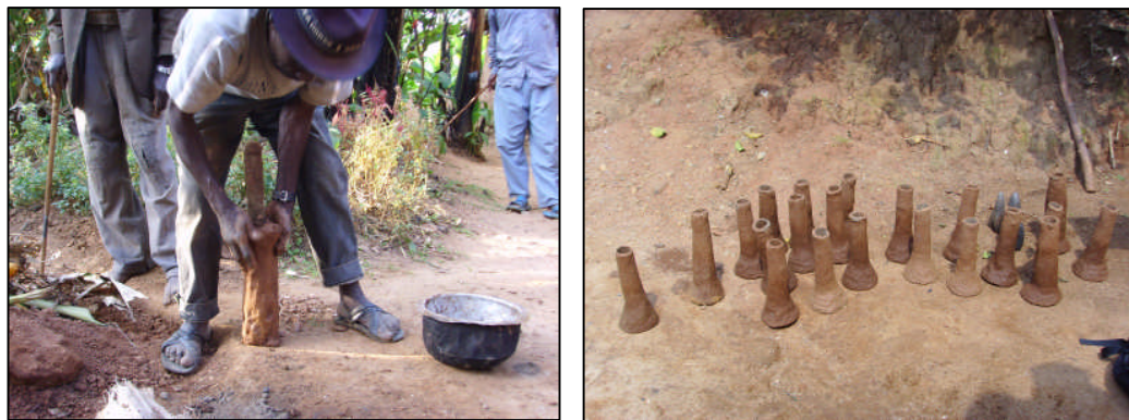
Fig. 2.2 Tuyere production (left), and the finished products (right)
