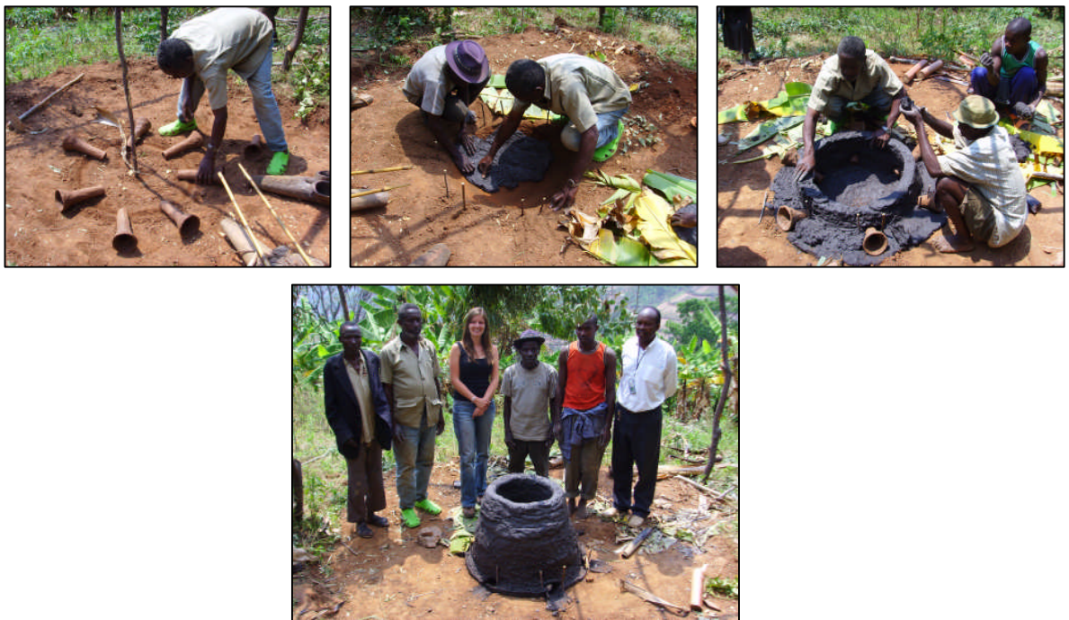
2.5 Constructing the furnace: laying out the tuyeres (top left), lining the furnace pit (top middle), building up the superstructure (top right), the finished furnace structure and the team (bottom)
