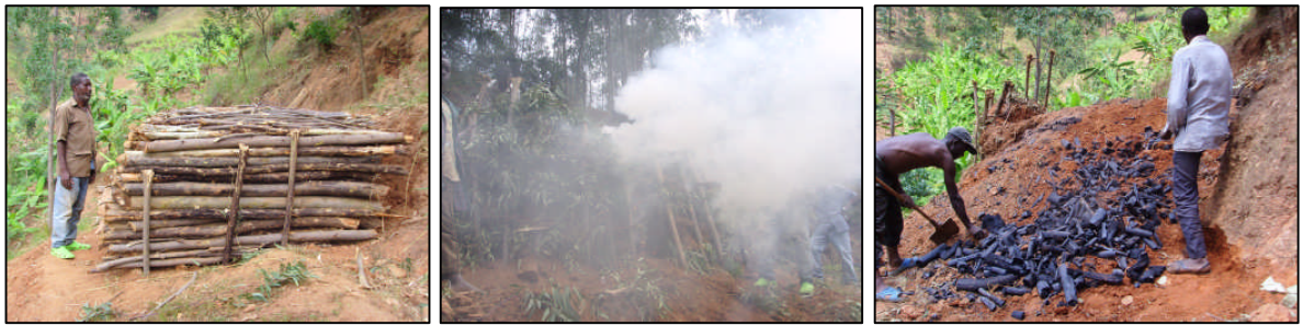
Fig. 2.1 Charcoal production: the wood stacked (left), slowly combusted (middle), and the charcoal revealed (right)
