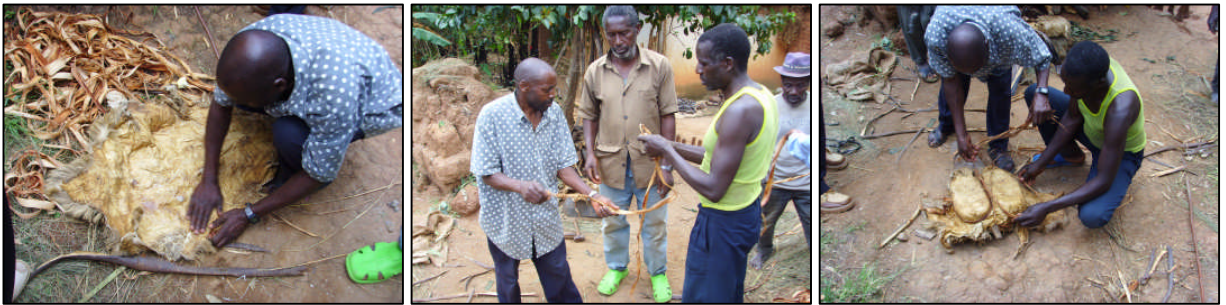
Fig. 2.3 Assembling the bellows: greasing the skins (left), preparing the rope (middle), and attaching the skins (right)
