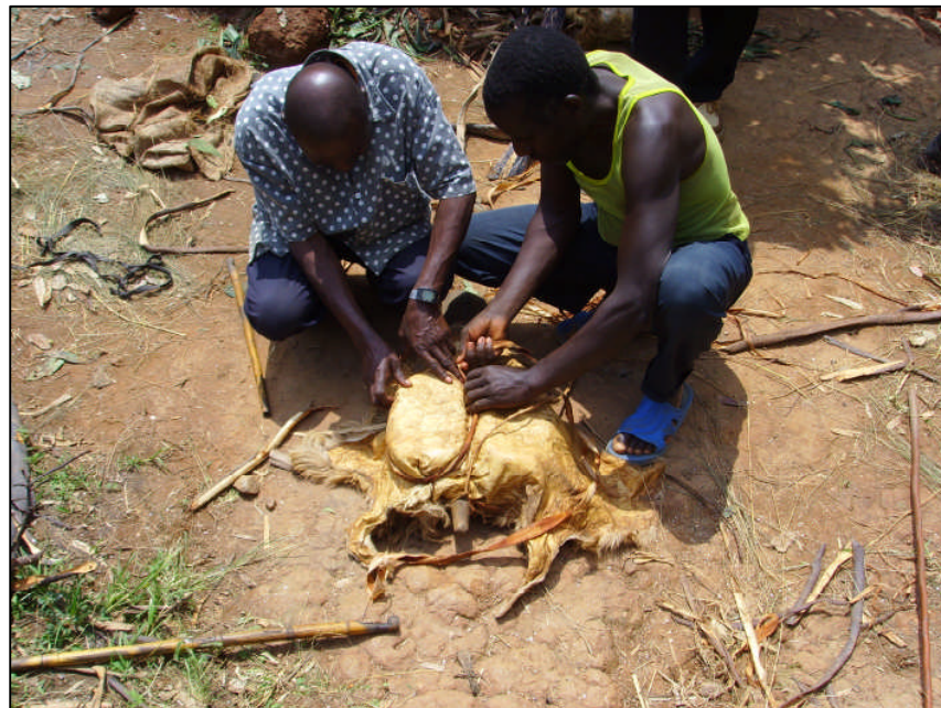
Fig. 3.3 Members of the smelting group commissioned in Rwanda, attaching sheep skins to wooden bellows
