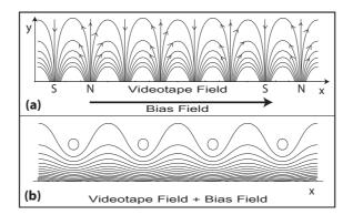
Figure 1. (a) Videotape magnetic field lines and uniform bias field. (b) Contours of constant field strength once the bias field is added. Weak-field-seeking atoms can be trapped in the circular minima.
