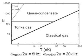
Figure 2. Number of atoms in the 1D system versus temperature in nanoKelvin for different values of the radial  $(\omega_{radial})$  and axial  $(\omega_{axial})$  frequencies of the trap, for  $^{87}$ Rb. Three quantum regimes can be found below the degeneracy temperature: a "quasi-condensate", a pure condensate and the Tonks-Girardeau gas. The gas behaves classically to the right of the degeneracy line.
