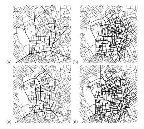
Figure 6: (a) and (b) Weighted mean depth for a  $3\text{km} \times 3\text{km}$  axial system. Thicker lines have lower values (i.e., thicker lines are more central). (a) shows angular mean depth; (b) shows block-distance mean depth. (c) and (d) Weighted mean depth for the road-centre line map of the same area. (c) shows angular mean depth; (d) shows block-distance mean depth. Base map data ©Crown Copyright/database right 2005. An Ordnance Survey/EDINA supplied service.
