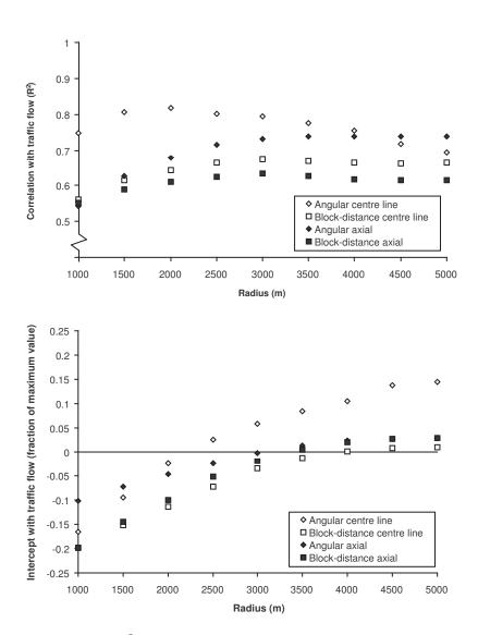
Figure 8: (a)  $R^2$  correlation coefficients and (b) intercept values for best fit lines of vehicular flow against weighted choice (for both axial and road-centre line maps and block-distance and angular measures).
