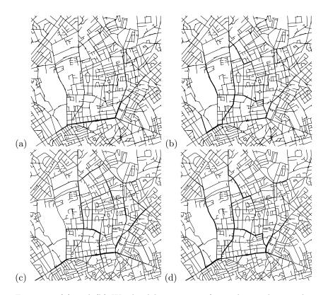
Figure 5: (a) and (b) Weighted betweenness for a  $3 \text{km} \times 3 \text{km}$  axial system. Thicker lines have higher values. (a) shows angular betweenness; (b) shows block-distance betweenness. (c) and (d) Weighted betweenness for the road-centre line map of the same area. (c) shows angular betweenness; (d) shows block-distance betweenness. Base map data ©Crown Copyright/database right 2005. An Ordnance Survey/EDINA supplied service.
