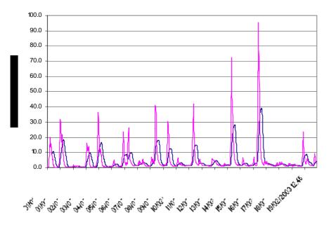
Figure 1: Carbon monoxide measurements from a home with a problem gas fire (House number 447374). The lighter line is the 15-minute average data, the darker smoothed line is the 8 hour moving average value.
