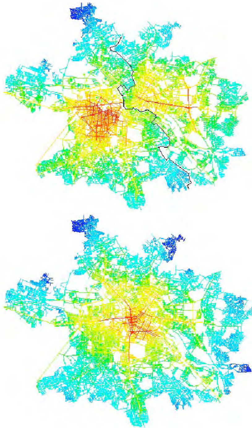
Figure 6.4 Axial analysis of Berlin before and after unification, showing the relocation of the integration core (higher integration values shown moving from blue, through green, yellow and to red) [Source: Desyllas, 1998].
