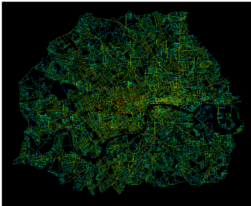
Figure 5.1 The top two figures demonstrate how small changes in morphology represent significant configurational changes, expressed through the j-graph. The lower figure is an axial map of London, the summation of the individual j-graphs of every line in the system. The ‘hotter’ colours indicate higher integration, that is fewer ‘steps’ to every other line in the system.
