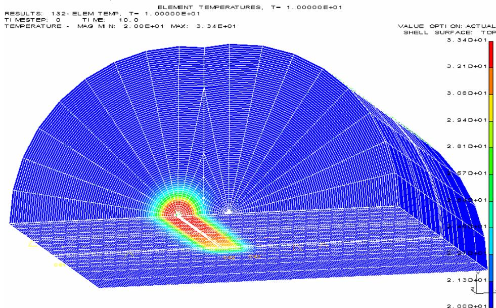
**Figure 2. Temperature contour plot for the 3D FE model at 10 seconds**
