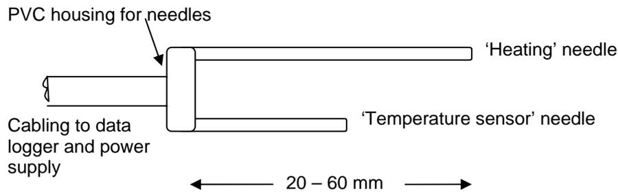
**Figure 1. A conceptual dual-probe (not to scale)**
