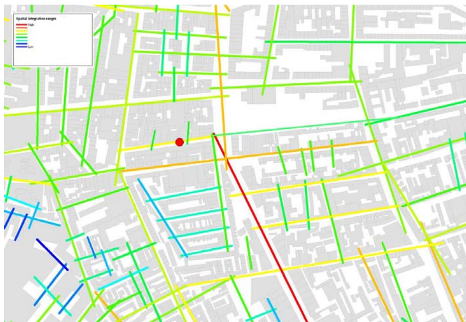
Space syntax map showing distribution of integration from red (integrated) to blue (segregated) in the vicinity of Dorset Street
