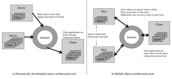
Figure 1: Two architectural styles for distributed OO software
