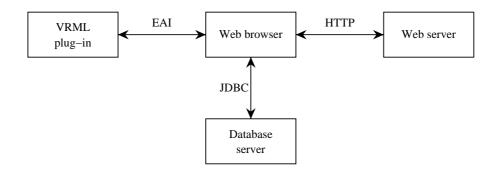
Figure 2: 3DSoftVis: Physical structure.
