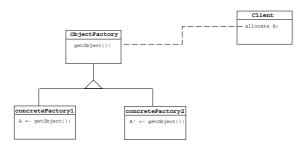
Figure 2: Semi-Dynamic Configuration: Instantiation Factories
