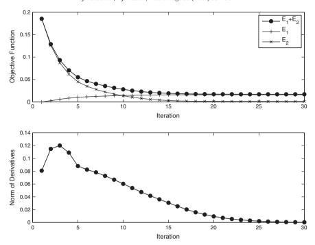
**Fig. 3.** Convergence of the Gauss–Newton optimisation. The top panel shows how the objective function is reduced at each iteration, whereas the lower panel shows the norm of the derivatives of the objective function with respect to the model parameters. At the exact solution (either globally or locally optimal), this norm should be zero.
