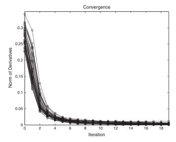
**Fig. 13.** The norm of the derivatives of the objective function after different numbers of Gauss–Newton iterations. In principle, the norm should be zero if the algorithm has fully converged.
