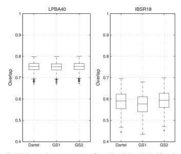
**Fig. 7.** Volume overlap measures compare favourably with those obtained from the other registration algorithms evaluated in Klein et al. (2009) (this figure may be compared directly with Fig. 5 of that paper). On each box, the central mark is the median, the edges of the box are the 25th and 75th percentiles, the whiskers extend to the most extreme data-points not considered outliers. Any outliers are plotted individually.
