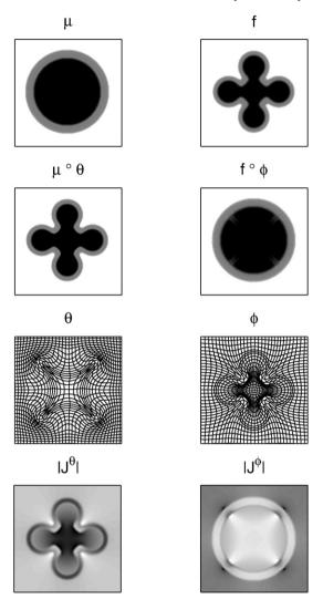
**Fig. 2.** Results of diffeomorphic registation of two simulated images. Original images (top row), registered images (2nd row), diffeomorphic deformations (3rd row) and Jacobian determinants (bottom).
