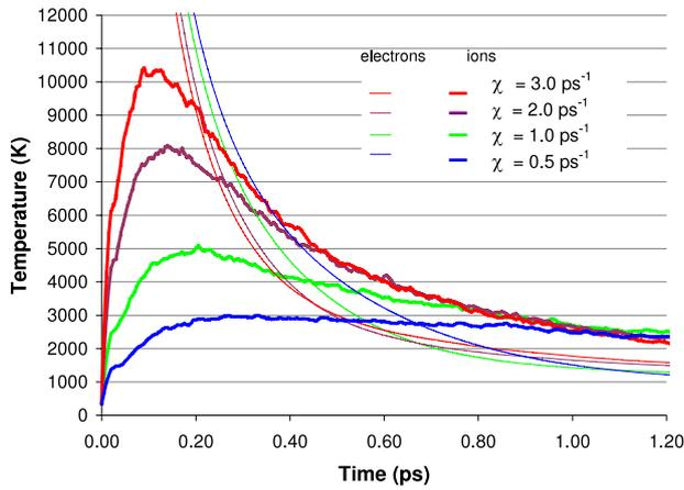
**Figure 2.** Time evolution of  $T_l$  (thick lines) showing lattice heating till about 0.2 ps, heat diffusion for the next 0.4 ps, and electron–lattice energy exchange for the remainder of the simulation. The corresponding evolution for  $T_e$  is shown by thin lines.
