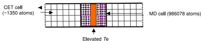
**Figure 1.** Schematic representation of the simulation cell. The swift heavy ion travels vertically through the centre of the cell. The thick black lines represent periodic boundary conditions and the dotted lines represent constant electronic temperature ( $T_e$ ) boundary conditions. The number of coarse-grained electronic temperature (CET) cells has been reduced for clarity.
