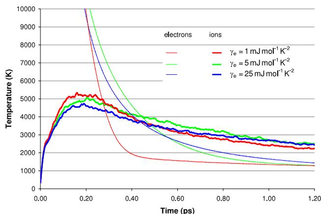
**Figure 4.** Time evolution of  $T_i$  (thick lines) and  $T_e$  (thin lines) for the first 1.2 ps of simulations for 3 values of the electronic specific heat coefficient ( $\gamma_e$ ). Note the rapid decay of  $T_e$  for low  $\gamma_e$ , resulting in faster cooling of the lattice.
