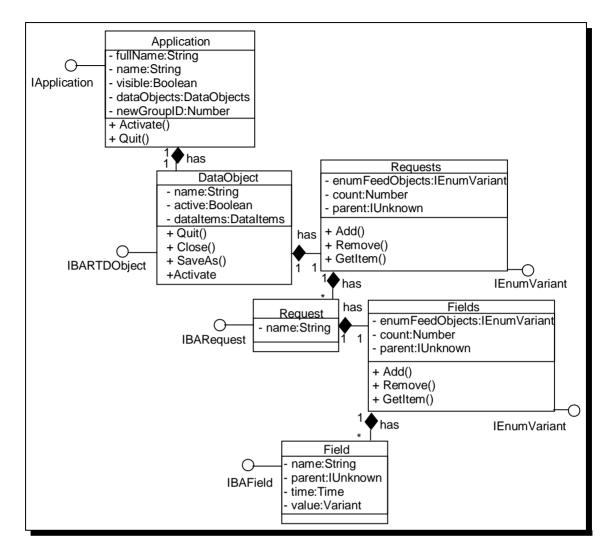
Figure 4: Object Model for Filter Component
