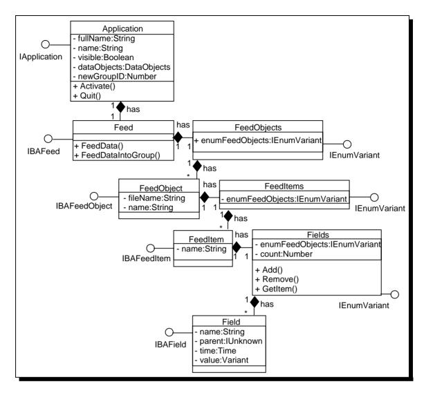
Figure 3: Object Model for Input Component
