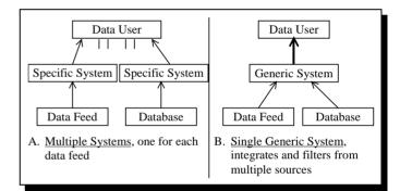
Figure 1: Multiple vs Single Feed Processor
