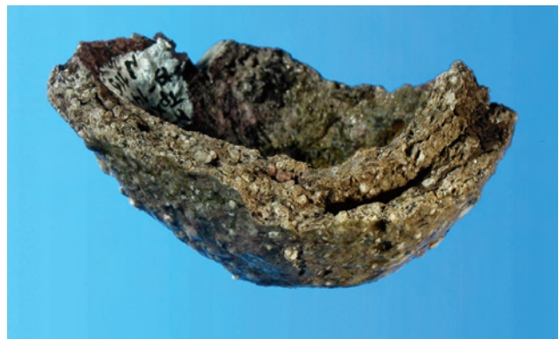
Figure 2 Early medieval bronze-melting crucible from Novgorod, Russia. It is made from refractory clay tempered with quartz to improve its thermal performance and has been heated from below/outside. Wall thickness 6–10 mm.
