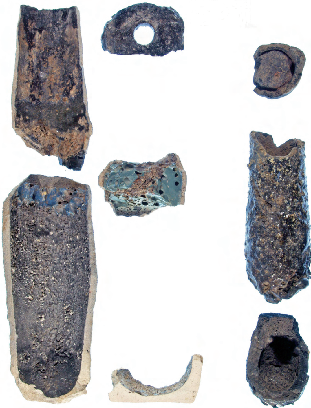
Figure 10 Typical steel-making crucibles from 11th-century Akhsiket, Uzbekistan (left and centre) and 19th-century Sri Lanka (right); both are lidded. The Uzbek crucibles are made from white-firing dense kaolinitic clay tempered with quartz sand, are c. 300 mm tall and c. 80 mm wide internally, and have a small opening in the lid. The Sri Lankan crucibles are about 200–250 mm total length and c. 30 mm wide internally. Their ceramic is black and porous due to a high amount of rice husk temper, and their lids are pierced with a few hair-fine vents.
