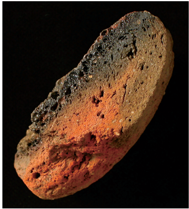
Figure 1 Cross-section through the rim of a Late Bronze Age bronze-melting crucible from Qantir-Piramesses, Egypt. It is made from non-refractory Nile silt and heated from above/inside, resulting in extensive vitrification and bloating of the ceramic. Wall thickness c. 20 mm.
