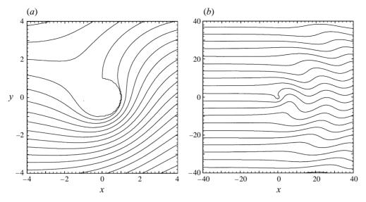
FIGURE 3. Contours of  $\psi + uy$  for a cyclone for (a)  $-4 \le x, y \le 4$  (contour interval of 0.5) and (b)  $-40 \le x, y \le 40$  (contour interval of 3.5). In each case b = 1/3 (u = -0.9) and a = 1.
